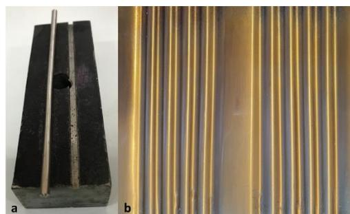
Fig. 1. a) Construction devise for electrode A and b) electrode A.
