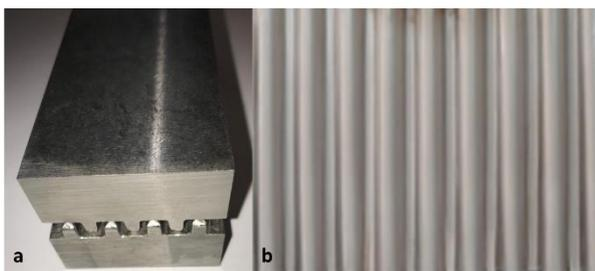
Fig. 2. a) Matrix for machining electrodes and b) electrode B.
