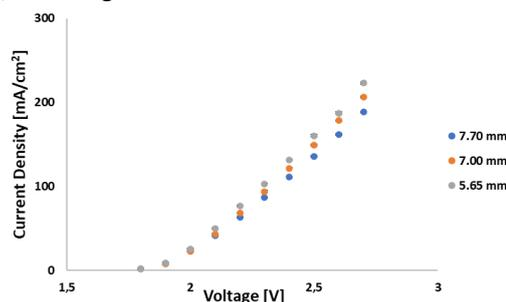
Fig. 3. Polarization curves at different distances between electrodes A.
