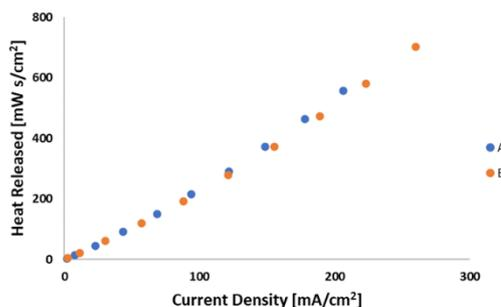
Fig. 6. Energy released in the production of hydrogen and oxygen at the same current density for electrode A and B.
