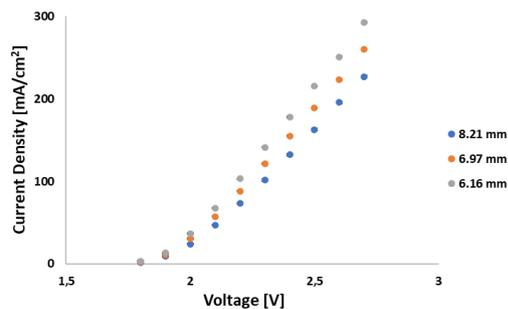
Fig. 4. Polarization curves at different distances between electrodes B.
