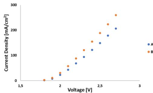
Fig. 5. Polarization curves of electrode A at 7.00 [mm] and electrode B at 6.97 [mm].
