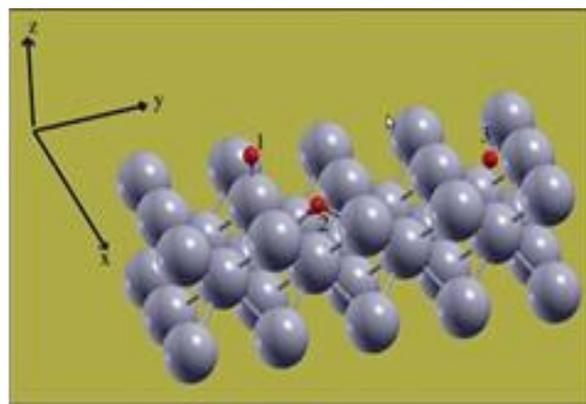
Figure 1: Scheme of the considered system W-atom: (1) top, (2) bridge, (3) hollow interaction sites.
