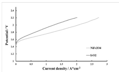
**Figure 1** Linear sweep voltammeteries for the cells based on NiFe<sub>2</sub>O<sub>4</sub> hollow spheres and IrO<sub>2</sub> at the anode.
