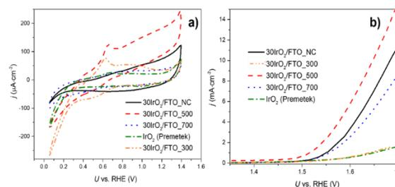
Fig. 1. OER characterization of  $\text{XIrO}_2/\text{FTO}_Y$  in RDE setup by means of a) CVs retrieved at  $20 \text{ mV}\cdot\text{s}^{-1}$  and b) OER LSVs recorded at  $2 \text{ mV}\cdot\text{s}^{-1}$  in an Ar saturated 0.1 M  $\text{HClO}_4$  solution at  $25 \text{ }^\circ\text{C}$ . The loading of Ir catalyst was kept at  $14.2 \mu\text{g}_{\text{Ir}}\cdot\text{cm}^{-2}$  in the  $0.196 \text{ cm}^2$  Au WE tip at 1600 RPM.
