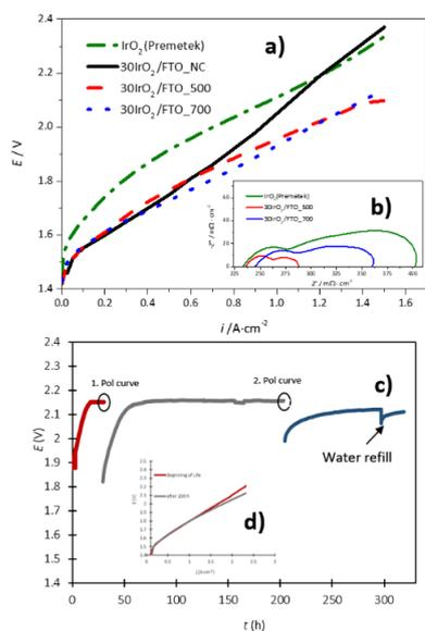
Fig. 2. PEMWE performance and stability using IrO<sub>2</sub> and 30IrOx/FTO\_Y (NC/500°/700°) CCM anodes in a cell with N117 at 60 °C); b) EIS recorded at 2 A·cm<sup>2</sup>; c) long-term chronopotentiometry at steady 1000mA·cm<sup>2</sup> d) Pol curves recorded at BoL and after 200 h of operation @ 75 °C.
