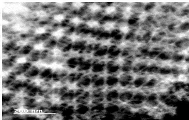
**Figure 1** TEM images of 3DOM Mn<sub>0.5</sub>Ni<sub>0.5</sub>Co<sub>2</sub>O<sub>4</sub> Electrocatalyst
