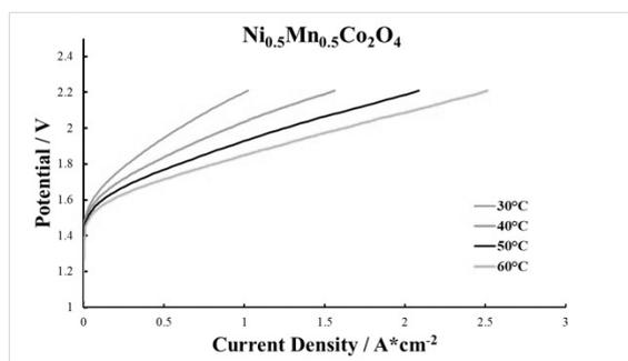
**Figure 2** Linear sweep voltammetry at different temperatures the MEA equipped with  $\text{Mn}_{0.5}\text{Ni}_{0.5}\text{Co}_2\text{O}_4$  anode catalyst.
