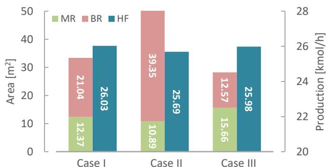
Fig. 2. Reactor areas (MR and BR) and hydrogen production (HF) after process optimization for the three cases under study.
