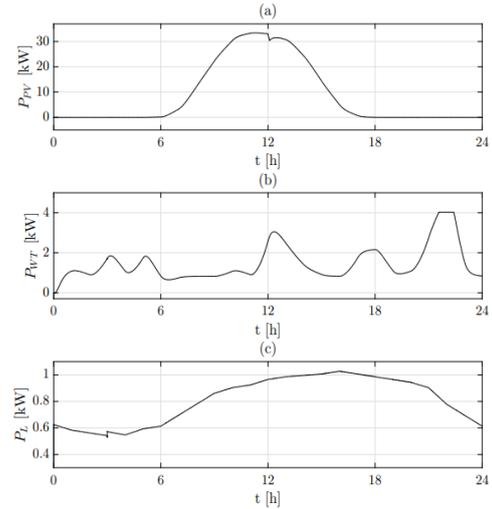
Fig. 3 24 hours profiles of: (a) Power irradiance, (b) Power of wind turbine and (c) Load power consumption.
