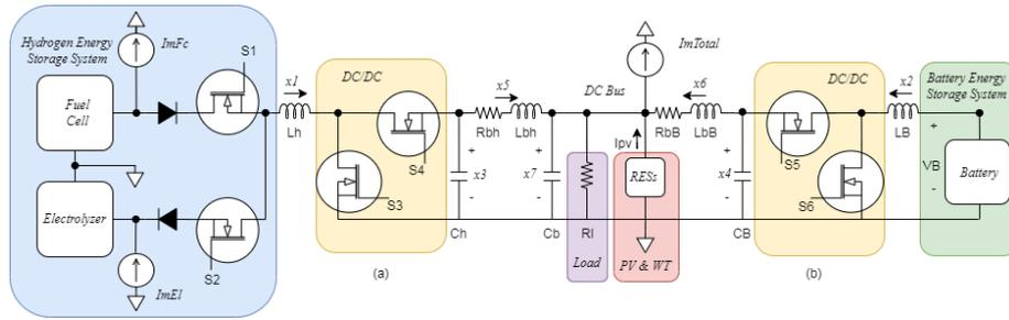
Fig. 2 Electrical diagram with the variables involved of the MG.
