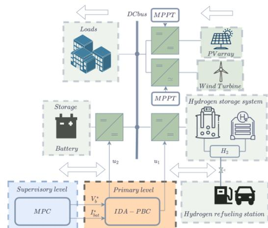
Fig. 1. Isolated DC MG scheme with a typical structure of electric-hydrogen hybrid refueling station.
